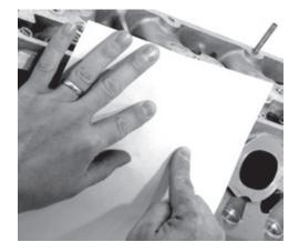
Place a sheet of paper covering port(s). Holding it firmly with one hand, use your index finger to rub the edges of the port(s) and bolt holes.
