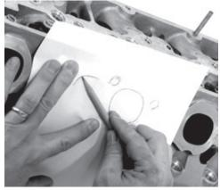
Holding the pencil's face flat against the paper, define the ports and bolt pattern.
