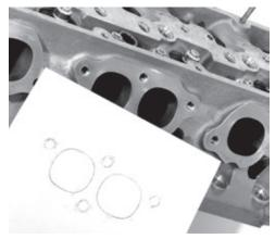
Make sure the transfer is accurate and the paper did not slip during the process.
